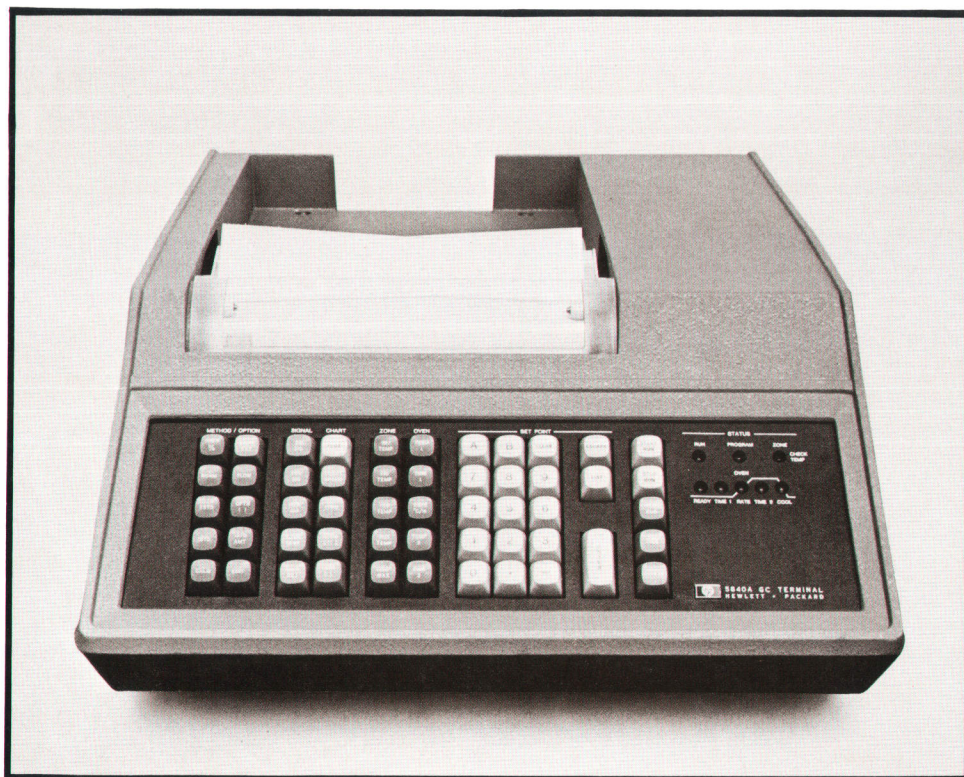
Fig. 5. Through the keyboard, all aspects of the analysis are controlled—the column oven temperature program, the temperatures of other heated zones, the integration parameters, the calibration, and the type of computation. Operation of backflush valves, a change in recorder speed, a change in detectors, and other parameters can be programmed to occur at specific times following the start of a run.
